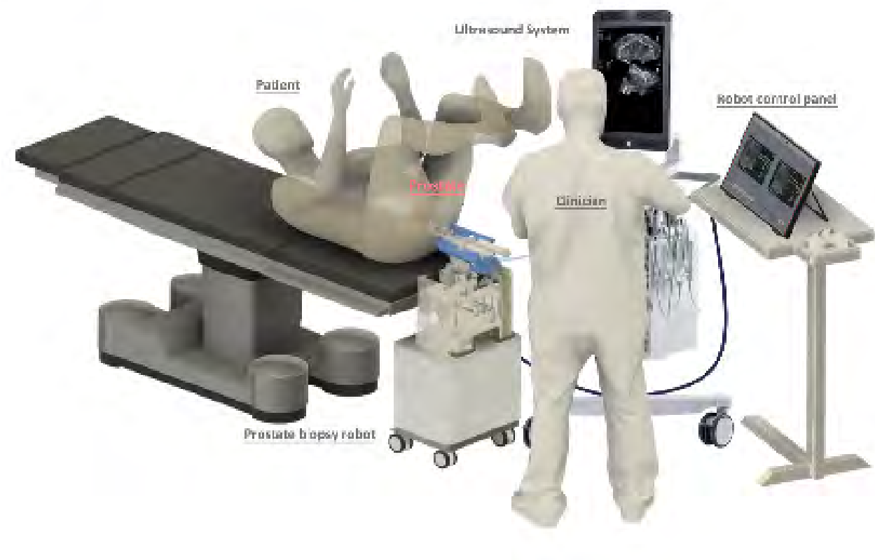
Illustration of the designed robotic prostate biopsy system with BK ultrasound system equipped with bi-planar transducer.
